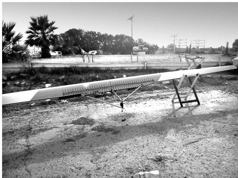
Picture 1 - Boat with footage: to calculate the amplitude
